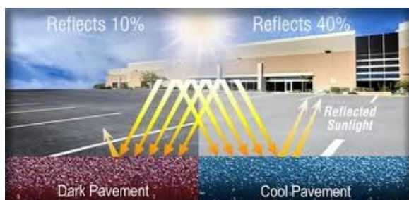
Figure 7. Dark Pavement versus Cool Pavement sunlight reflection.
